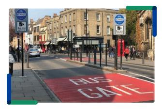
A Bus Gate is a sign-posted short length of stand-alone bus lane. This short length of road is restricted exclusively to buses, taxis and cyclists plus emergency vehicles. It facilitates bus priority by removing general through traffic along the overall road where the bus gate is located. General traffic will be directed by signage to divert away to other roads before they arrive at the bus gate. To see an animation of a how a Bus Gate will work, please visit our website www.busconnects.ie.
